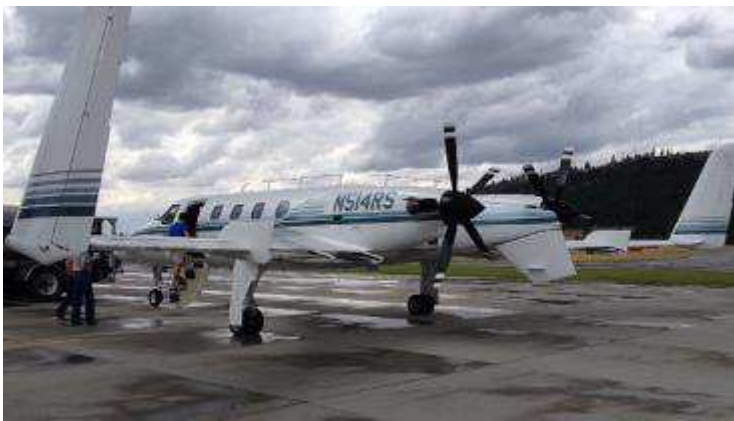
Notice the Canard in front and the "Pusher" propeller in back.
