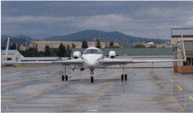
Notice the Canard in front and the "Pusher" propeller in back.
